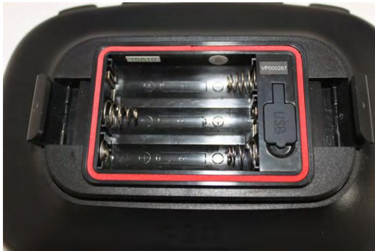
**Figure 2.** Gasket Channel Location
