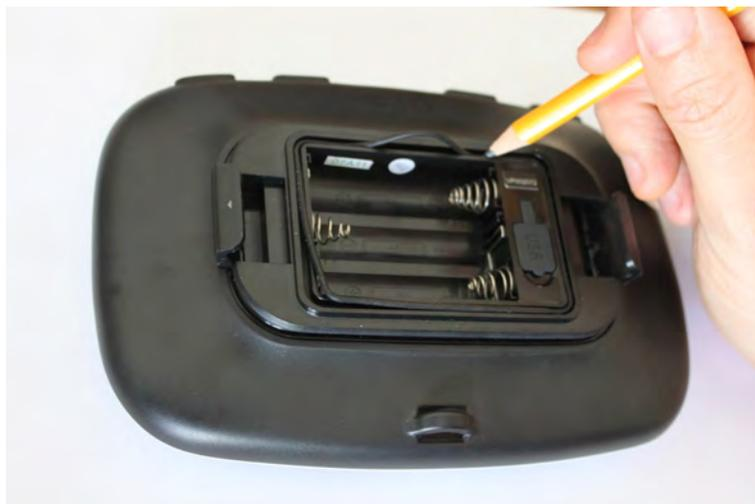
**Figure 3.** Causing Gasket to Buckle
