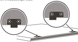
Attach the tail panel to the stationary panel by angling it 90° from the bed rails, sliding its driver-side, slip joint hinge together, then dropping its passenger-side, drop-on hinge together.
