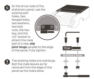
Repeat step 5 on the passenger side of the center panel using the male half of a drop-on hinge.
