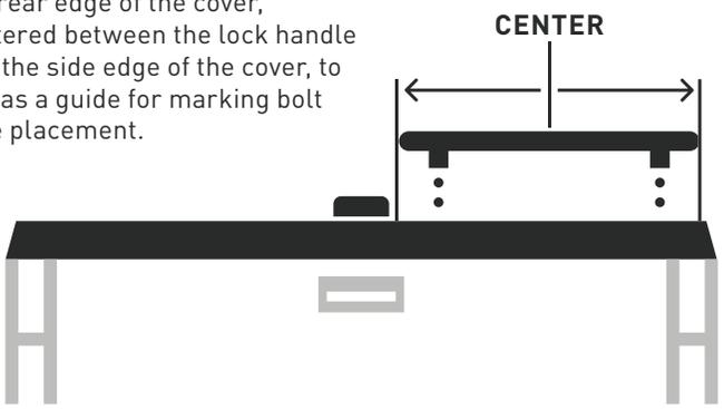
**2** Measure 3/4" from the rear edge of cover to mark hole placements in line with the adapter-bar bolts.
