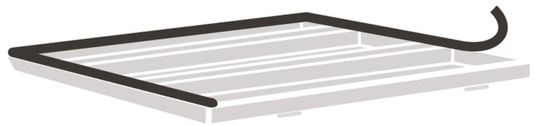
5. Cut off the excess weatherstrip. Close and lock the cab panel. Leave it closed for 24 hours to allow the weatherstrip adhesive to cure.
