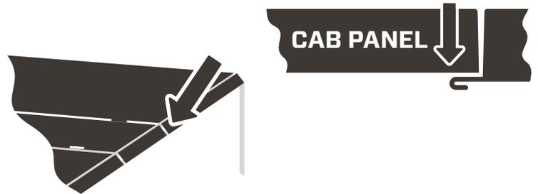
2. Open the cab panel. Remove the original weatherstrip from the flange.
