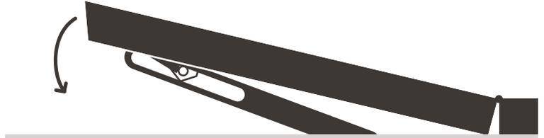
2. Push up on the safety catch so its triangle clears the ball stud. Push the cab panel up.
