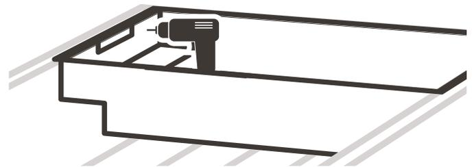
**5** If you just installed the bin under a DiamondBack cover you've had for a while, you may find that your cab-panel lock rods are now more difficult to operate. If so, use the rod guide brackets and a 7/16" socket to lower the rods slightly.
