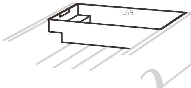
**★** Many pickup truck cargo beds are tapered, which means that many Cross Bins have a front and back. Look for the word "CAB" etched into one of the longer inside walls of the bin; make that wall the one nearest the cab.
