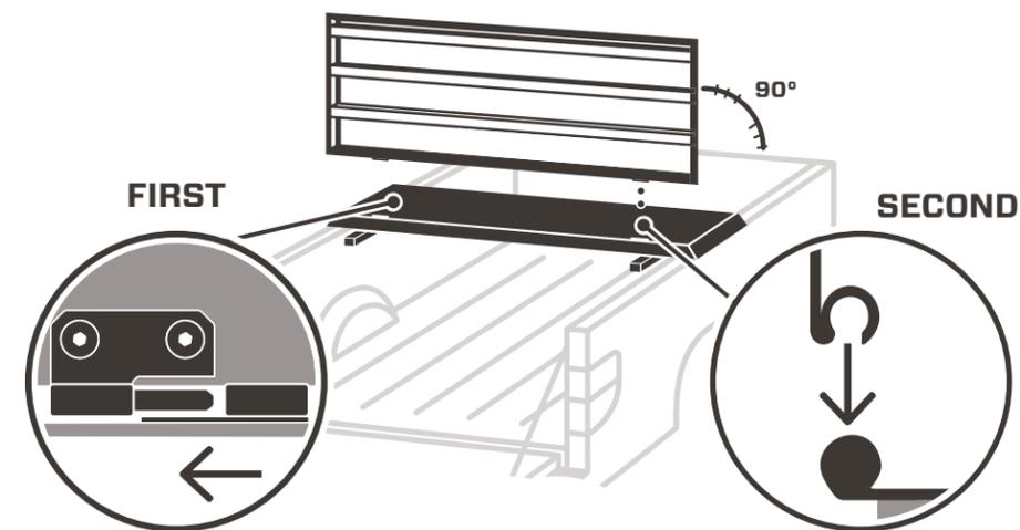
**!** To avoid hinge damage, make sure the C-shaped hinge knuckle is fully engaged with its pin before tilting the panel.
