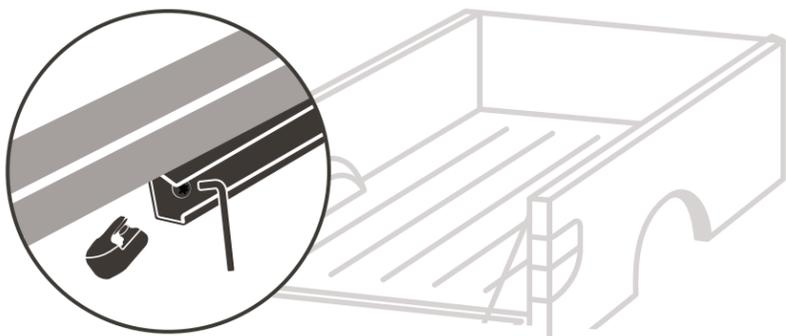
**3** Slide the driver-side **lock-rod striker bracket** into the deck rail until its forward hole aligns with the factory bolt.
