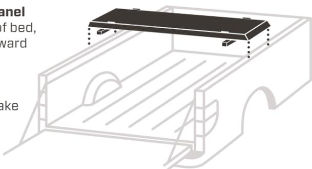
**7** Attach the **tail panel** by angling it 90° from the bed rails, sliding its driver-side, loop-shaped hinge knuckle fully onto the corresponding center-panel hinge pin, then dropping its passenger-side, C-shaped hinge knuckle fully onto its corresponding pin.
