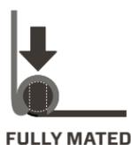
**3** Lower the tail panel into the closed position.
