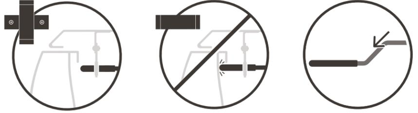
**15** With the lock handle in the closed position, position the lock rods tight against the underside of the striker brackets so that they'll draw the panels down and compress the weatherstrip. Tighten the rod guide brackets with a 7/16" socket.
