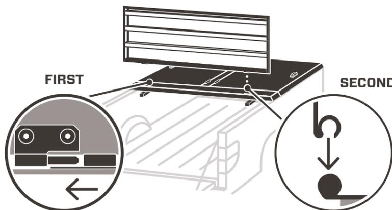
**8** Lower the tail panel into the closed position.
