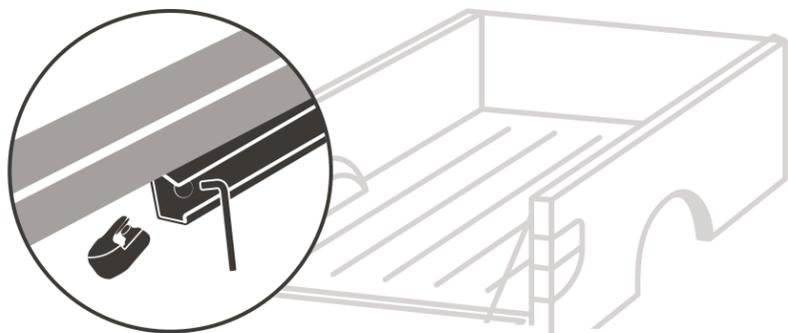
**3** Slide the driver-side **lock-rod striker bracket** into the deck rail until its forward hole aligns with the factory bolt hole.
