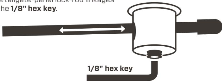
**14** Adjust the length of the lock rods and retighten the set screws so that:
