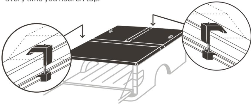
**13** Close the tail panel. Loosen the set screws on the tailgate-panel lock-rod linkages with the **1/8" hex key**.
