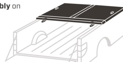
**7** Attach the **tail panel** by angling it 90° from the bed rails, sliding its driver-side, loop-shaped hinge knuckle fully onto the corresponding center-panel hinge pin, then dropping its passenger-side, C-shaped hinge knuckle fully onto its corresponding pin.
