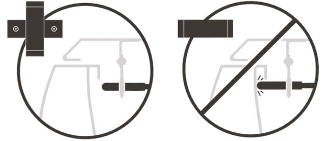
**15** With the lock handle in the closed position, position the lock rods tight against the underside of the striker brackets so that they'll draw the panels down and compress the weatherstrip. Tighten the rod guide brackets with a 7/16" socket.
