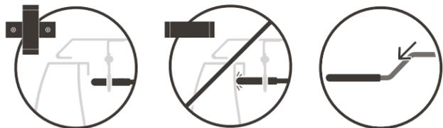
**30** Position the lock rods tight against the underside of the bed rails so that they'll draw the panels down and compress the weatherstrip. Tighten the rod guide brackets with a 7/16" socket.
