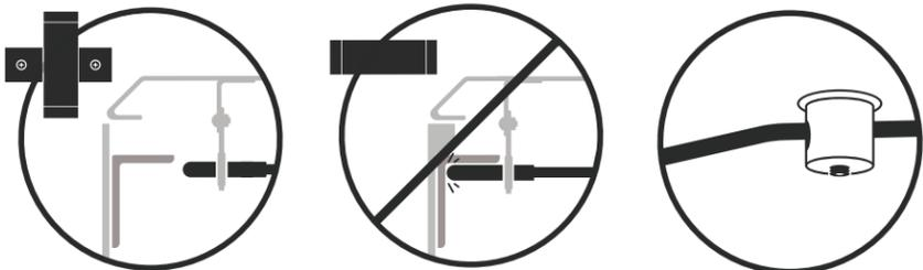
**24** With the lock handle in the closed position, set the lock rods tight against the underside of the bulkhead angle. Tighten the rod guide brackets with a 7/16" socket.
