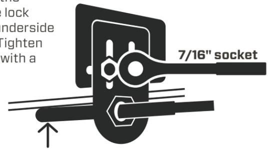
**25** Double-check both panels to ensure they open, close, lock & seal correctly. If at any point the weatherstrip does not touch the bed rails, readjust the lock rods and mounting brackets as needed.
