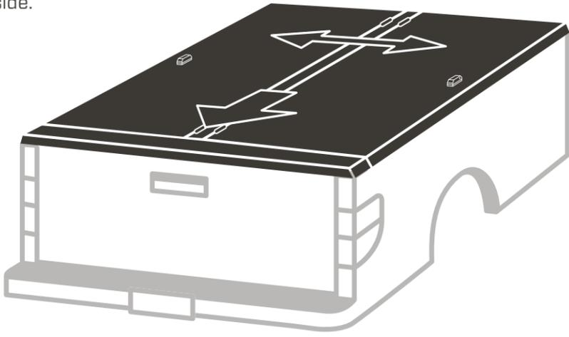
**20** Attach the nose of the T panel to the bulkhead angle using two **cap clamps**. Tighten the clamps with a 9/16" socket.
