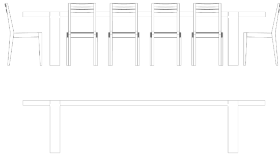
10 Seater (S) 3400 x 1000 x 750mm high | chairs 450mm wide Overhang: 450mm c/c
