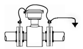
Install the MAG meter and connect the inlet and outlet to a proper GROUND line. This is the Solution Ground, called SG, and is very important for a stable ZERO FLOW measurement.
