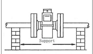
Install so that the meter is supported and not causing stress on the flanges.
