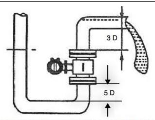
Install so that the meter is located so the outlet is at least 3 Pipe Diameters from any obstruction or elbow and the inlet is at least 5 Pipe Diameters and the meter is always submerged and there are no air bubbles
