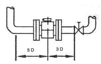
Install so that the meter is located so that the outlet is at least 3 Pipe Diameters from any obstruction or elbow and the inlet is at least 5 Pipe Diameters and the meter is always submerged and there are no air bubbles
