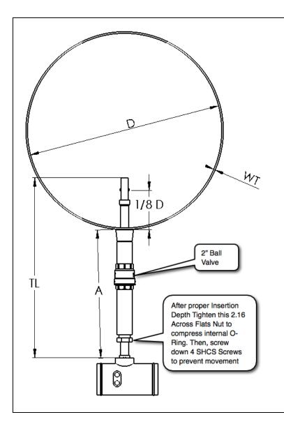
For clean water, the sensor may be placed at 1/8 of the inside diameter of the pipe.
