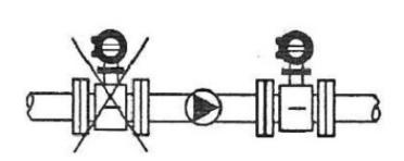
Do not install a MAG meter at the INLET of a pump as this will introduce bubbles. Instead, put it on the OUTLET with at least 5 diameters upstream.
