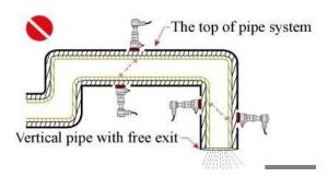
4. For locations with the flow exiting to ambient conditions the transducers should be installed on a U section of the pipe.
