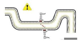
5. The temperature and pressure on the installation point should be within the specifications of the transducers.
