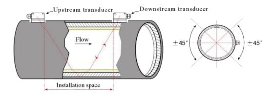
Use the Z method for large pipe diameters and where there may be suspended particulate or scaling. This method is ideal because the transducers transmit directly to each other without the reflection mode utilized in the V method. This method is known as the single sound path method.
