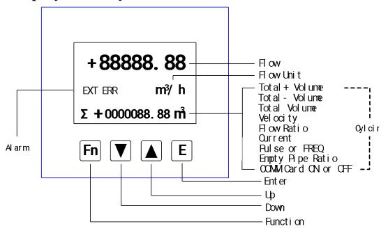
The electromagnetic flow electronics enters into the automatic measurement status after power on. All of the measurement functions are ready and measurement data is displayed.
