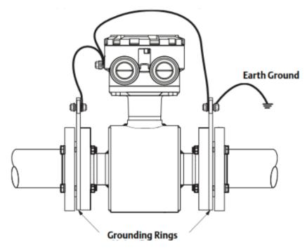
The MAG meter must be properly grounded for a stable reading. The grounding rings connect the ground to the fluid via the inner annulus of the grounding ring touching the fluid.
