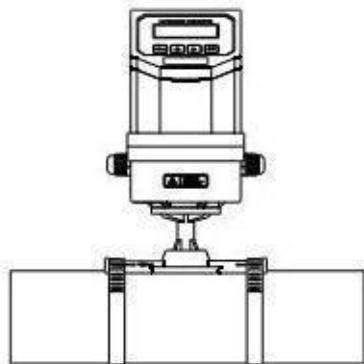
Install on the pipeline
