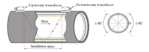
Use the Z method for large pipe diameters and where there may be suspended particulate or scaling. This method is ideal because the transducers dransmit directly to each other withoug the reflection mode utilized in the V method. This method is known as the single sound path method.
