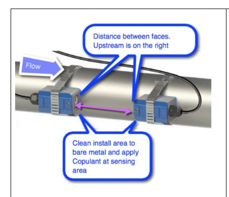
For pipes less than or equal to 6" we use SS Hose Clamps. The image shows where the transducers are held by the clamps. Put the transmitters on the SIDE of the pipe so sediment is not an issue. The SPACING on the Cheat Sheet is the distance you will measure between the FACES of the Upstream and Downstream transducers.
