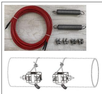
This is the clamping system for pipes larger than 10" OD. Install by securing ends with clamps WITHOUT the transmitter and then stretch the nylon coated SS wire over the transmitter. BE SURE to grind a CLEAN area for the transmitter to conduct the sound AND use the Acoustic Coupling Grease on the transmitter/pipe interface.
