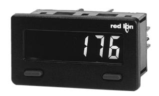
Programming notes. Hold SEL (Left BUtton) to start programming. Note: Press SEL many times to quit when done. Hold SEL to exit sub menus that allow selecting numbers for Scaling. Nice <u>video</u> showing 2 button User Interface.
