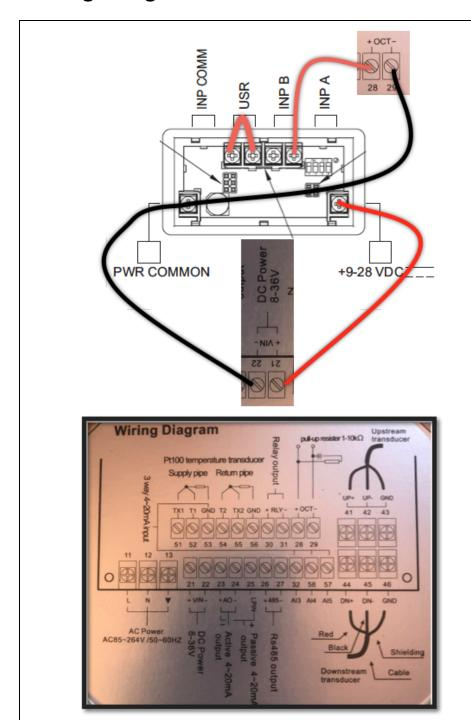
Note the small graphics show the actual connections and the larger graphic of the Ultrasonic Flow Meter gives the overall location of the connections.
