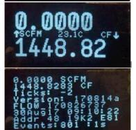
Sign On Screen. This screen only shows when the meter is powered on and is shown for 10 seconds during initialization of the meter
