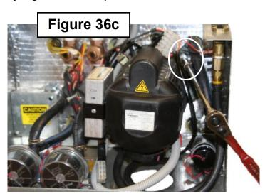
2. The eye-bolt nuts can then be tightened by using a 10mm socket wrench with a 10 inch long extension. Use extreme caution when tightening down the eye-bolt nuts, over tightening of the eye-bolt nuts can cause the aluminum blower casing to crack. (Torque Specifications = Approximately 20-40 in. lbs.)
