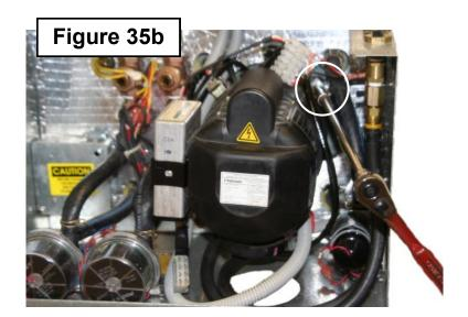
The Diesel-Burner is secured to the Hydro-Hot with two nuts that can be loosened, and swung out of the way by using a 10mm socket wrench with a 10 inch long extension.
