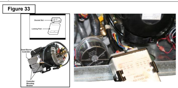
1. Locate the Diesel-Burner's Controller and disconnect both plugs.
