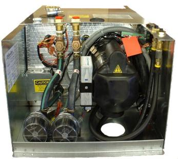
1. Locate the Diesel-Burner's Controller and connect both plugs.
