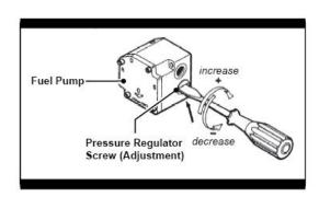
2. Once the fuel solenoid has been activated, and the fuel pressure gauge is registering a pressure, the fuel pressure can be adjusted. To increase the fuel pressure turn the pressure adjustment screw clockwise, and to reduce the fuel pressure, turn the pressure adjustment screw counter clockwise.
