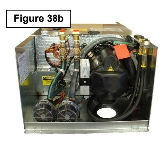
NOTE: The Diesel Burner's Controller might have to be mounted onto the side of the diesel burner, before the plugs are inserted into the control unit, otherwise it might not be possible to mount the control unit.
