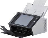
With the functionality of many devices, yet the simplicity of one, the N7100E network scanner contains the qualities organizations of all sizes desire to improve business processes. Scanning speeds are a consistent 25 ppm/50 ipm (A4 landscape 200/300 dpi) with a 50 sheet loading capacity.
