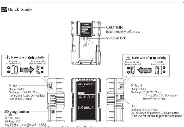
\* Red On: Error (Push and hold this button for 5 seconds)=>Reset
