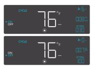
If there is a speed set in OFF Mode other than zero, the fans will run at that speed when triggered to turn off.
