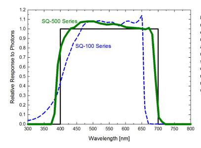
Mean spectral response measurements of six replicate Apogee SQ-100 and SQ-500 series quantum sensor. Spectral response measurements were made at 10 nm increments across a wavelength range of 300 to 800 nm in a monochromator with an attached electric light source. Measured spectral data from each quantum sensor were normalized by the measured spectral response of the monochromator/electric light combination, which was measured with a spectroradiometer.
