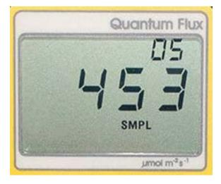
The LCD display consists of the total number of logged measurements in the upper right hand corner, the real-time PPFD value in the center, and the selected menu options along the bottom.
