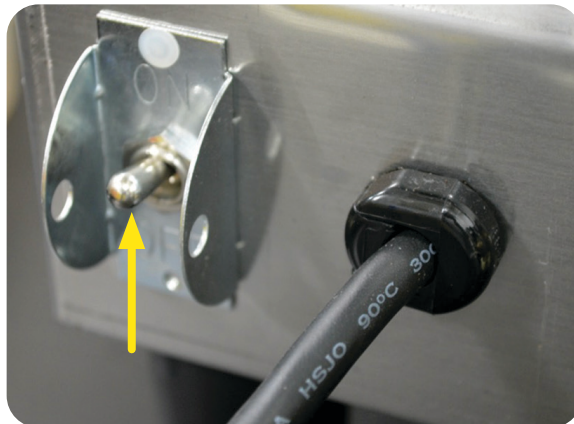
POWER SWITCH LOCATION
