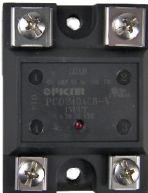
1.3740 - Solid State Low Voltage Relay, 40 amp. Used on Electrical Box Lids to Switch the Brew and Steam Elements.
