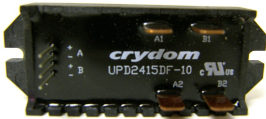
1.3752—Low Voltage Solid State Relay *Only For Machines After Serial Number xxxxx4080
