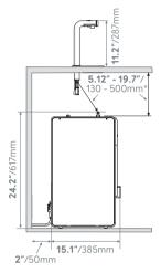
\* Hosing should be trimmed to ensure continuous drop from font to boiler
