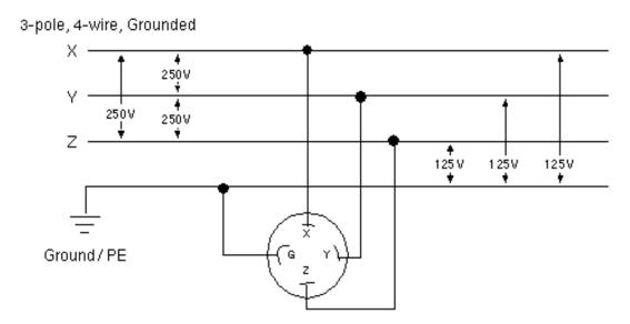
If your power is correct and the grinder operates but the rotational burr spins clockwise instead of counterclockwise, then you need to switch the position of any two hot lead wires, X, Y or Z (red, black, white) in the plug cap.
