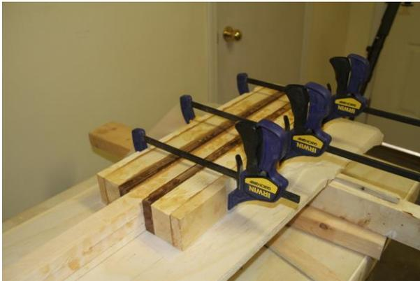
*Clamping blocks and shaft to form the basic blade structure.*
