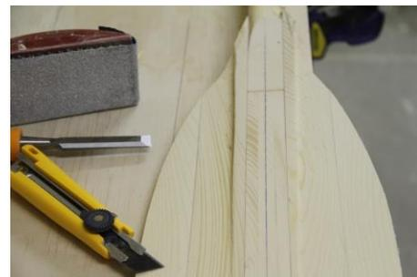
*Wood is removed from both sides of rectangle comprising upper spine.*
