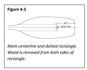
base can be used, however, this is not a common tool. Instead, a sharp half inch chisel can be used to efficiently remove wood to the required level. Be sure the chisel is very sharp, and as you get close to
