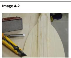
Wood is removed from both sides of rectangle comprising upper spine.
