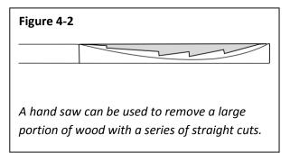
It is important the saw is sharp, and continually check both sides to make sure you don't cut below your pen line. When the angled saw starts getting too close (between 1/8" and ¼") to the pen line, make a vertical cut down from the top, and then begin another slanted horizontal cut. The vertical cuts are the ones you need to pay the closest attention to as the saw can remove wood quickly.
