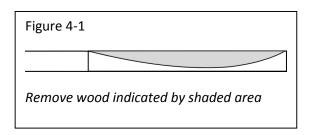
After scribing the curved line on both sides, the next step is to remove the wood above your pen line. Leave 1/8" wood above the line which will be removed later. There are several ways to remove the wood. A band saw with an 8" cut can be used (make sure you are fully comfortable using a band saw, as this is a tricky cut and you don't want to mess up at
