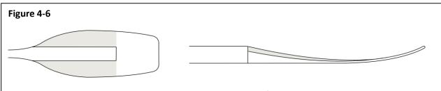
Shaded area indicates where wood is to be removed. Keep surface level and smooth as possible. Use flexible sanding block for final removal, and bring to  $1/8^{th''}$  from your line.
