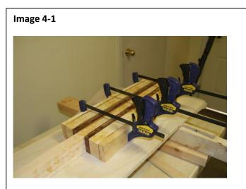
*Clamping blocks and shaft to form the basic blade structure.*
