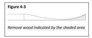
Removing the wood from this convex curve is much easier than the concave face on the top half. A hand saw or power tools can be used to remove a substantial portion of wood with a block plane used for cleaning up. Alternatively, if you're feeling energetic, a block plane (planing in the grain direction) can be used on its own to remove all the wood in
