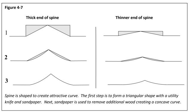
Make sure that the center line is clearly visible as you begin shaping the spine. Re-scribe if necessary. The first step is to use a sharp utility or carving knife to shave a triangular ridge as illustrated in figure 4-7. Pay extremely close attention to make sure you don't slice off the tip of the triangle, i.e. don't cut through the scribed center line. To ensure the sides of the triangle/ridge are even and fair, wrap a piece
