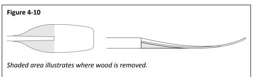
and sanding block remove the wood as illustrated in figure 4-10. Leave just under 1/8<sup>th</sup> proud. The edges of the spine can be rounded with utility knife and sandpaper to have a ½" radius (see fig 4-11)
