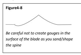
of 100 grit sandpaper around a tongue depressor and slide it up and down lengthwise. Be sure when you are sanding not to remove material too low, creating a gouge in the blade surface below (see figure 4-8).
