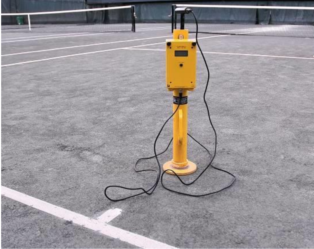
Photo 13: The Clegg Hammer is used to measure surface stiffness
