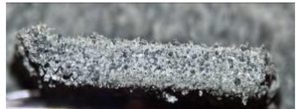
Photo 4: Magnified View of Compaction
