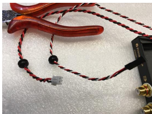
(10) Slide the rubbers over the wires
