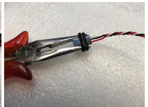
(9) Put the rubber over the black signal connector
