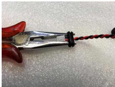
(8) Put the rubber over the white power connector
