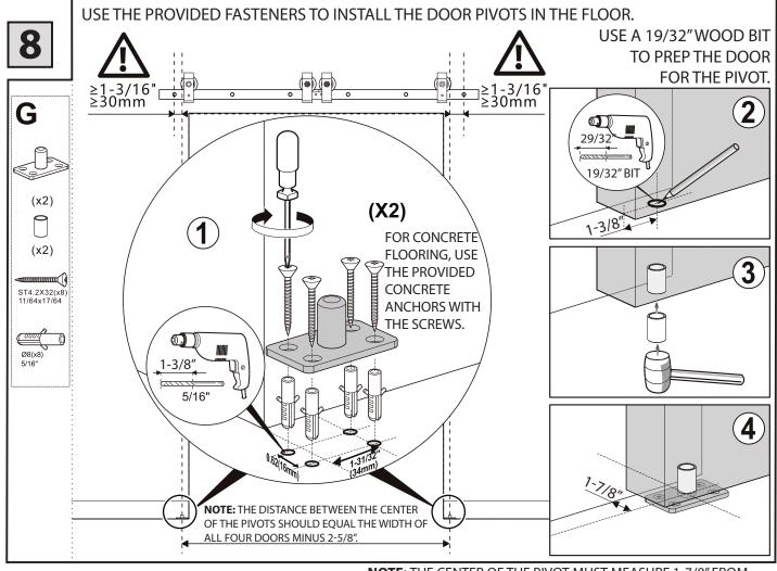
**NOTE:** THE CENTER OF THE PIVOT MUST MEASURE 1-7/8" FROM THE SURFACE OF THE HEADER BOARD WHERE TRACK IS MOUNTED.
