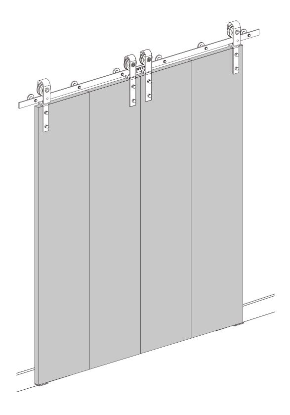
With proper installation, the maximum recommended weight for the folding door set is 176 pounds (44 pounds per panel). Sets will fit 1-3/8" - 1-3/4" thick doors.
