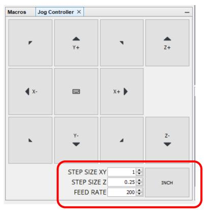
NOTE: The CNC will not jog –X, -Y, or +Z from the home position. This is because the Z axis is up as far as it will travel and The X and Y are as far back as the can travel.
