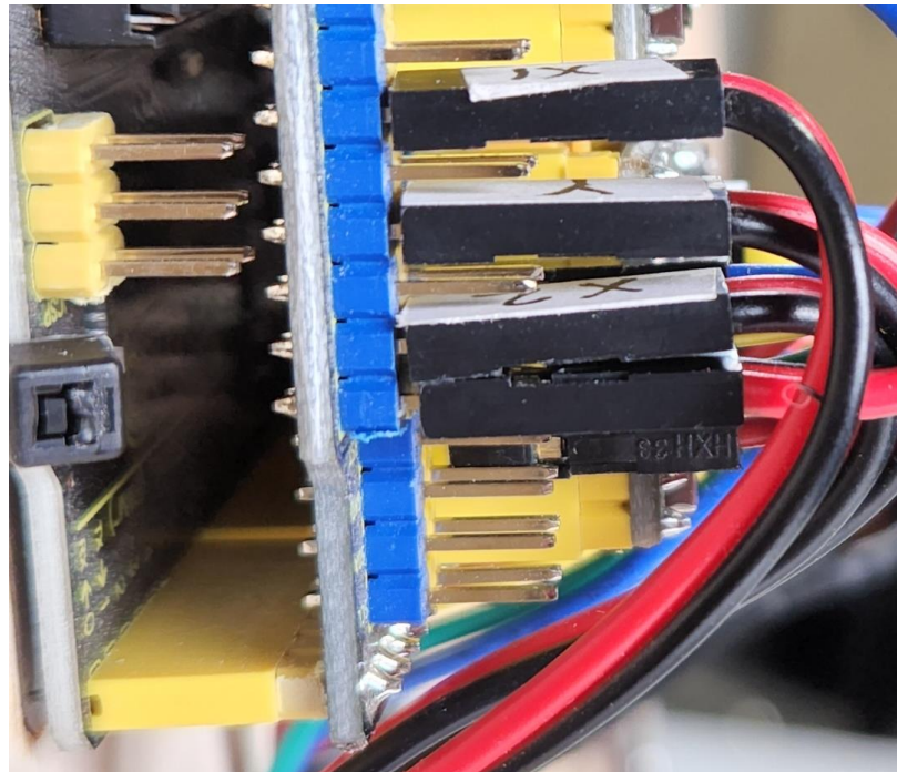
Side View of Home Switch Connections
