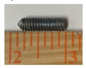
Hand turn the bolt into any of the threaded inserts in the bottom board and place your new spoilboard on top of the bottom board, making sure that you align it correctly. Then give the new spoilboard a little hand-pound above where you think the pointed bolt is located. That will create a small indent in the new spoilboard. Then move the pointed screw to the next hole. This is a very short process.
