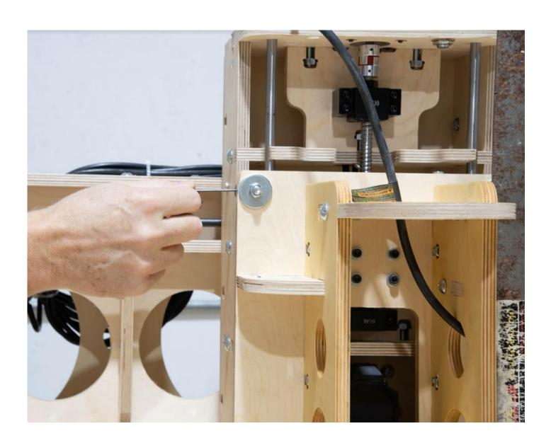
Step 3 Place the square as shown and look for a gap along the front of the Z Assembly.
