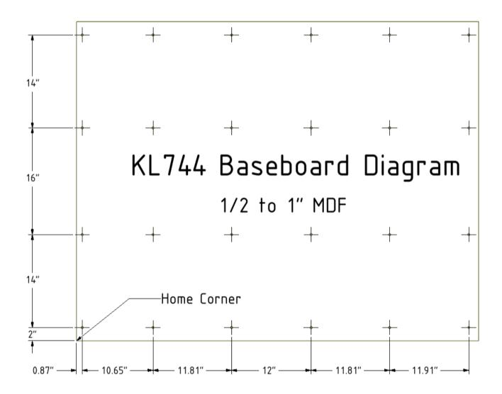
Step 2 Place the Baseboard into position so that the back side is flush with the X Frame Support.
