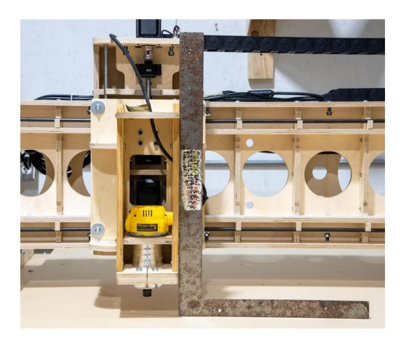
Step 2 Adjust the 4 SG25U bearings so that the gap closes and the side of the Z Assembly is parallel with the edge of the square.
