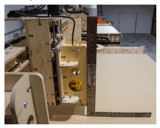
**Step 4** If needed, place the included Shim(s) in between the hub of the SG25U bearings and the fender washer on the Y carriage. Place matching shims on both of the top or the bottom bearings to rotate the YZ assembly clockwise or counter clockwise respectively.
