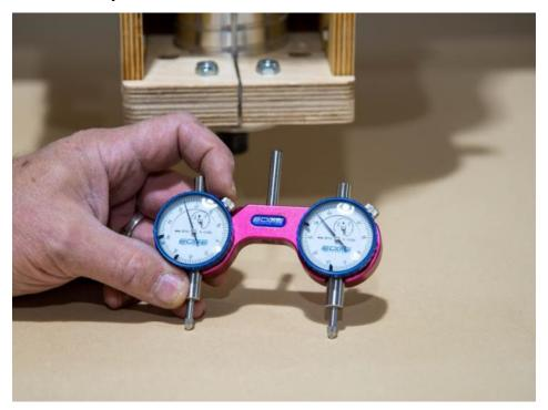
**Step 1** Insert the Tram Tool into the collet and snug the collet.
