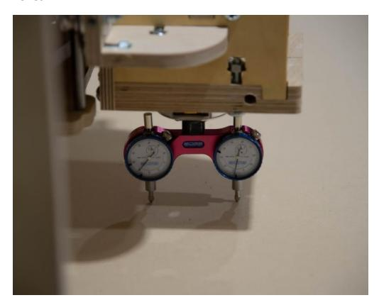
**Step 3** Adjust the 4 SG25U bearings to rotate around the X axis or install Shims to rotate around the Y axis until the dial indicator only moves a small amount. We recommend a total range of 0.002".
