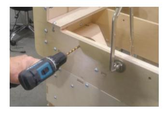
Step 3 Fasten the 1 x 3 Runner Boards with four 5/16"-18 x 1 3/4" Machine Screws and Nuts as shown.
