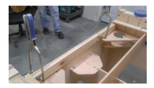
Step 2 Drill a 5/16" diameter hole into the Runner Board using the holes on the KL744 X frame holes as pilot holes as shown.
