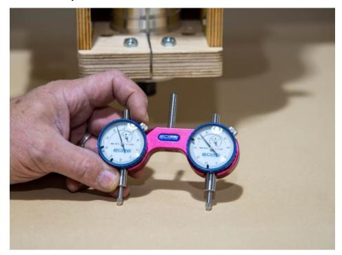
**Step 1** Insert the Tram tool into the collet and sung the collet.
