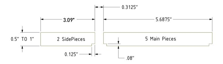
**Step 2** Lay out the MDF T-slots as shown and check ensure T-nuts freely slide and the end pieces align with the baseboard. NOTE: The two boards on the outside can be trimmed if needed to create the desired fit.
