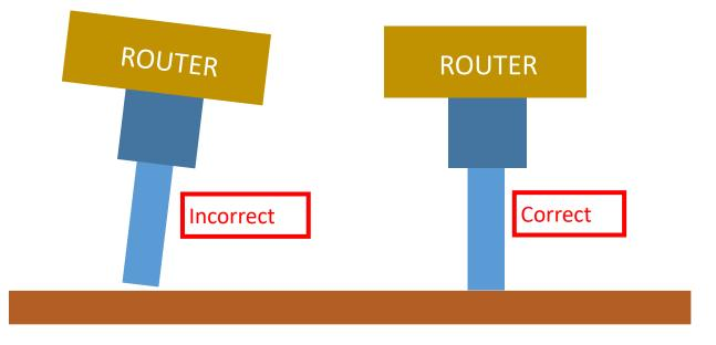
The KL7 Series routers have 4 SG25U bearings in slotted holes. There are 8-32 Set Screws that can be used to precisely move any of the 4 SG25U bearings to rotate the Z Assembly around the X axis so that it is perpendicular to the Spoilboard surface.
