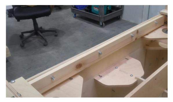
Step 4 Repeat Step 3 for the remaining four Runner Boards as shown. The back Runner Board should be mounted with the machine screw heads on the outside.
