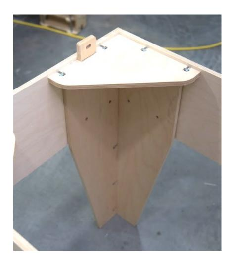
NOTE: The Mounting Tab on the End Leg Panels will fasten to the front and rear End Panels of the KL7 Series Router with four  $5/16 \times 1$  1/4 Machine Screws and Nuts .
