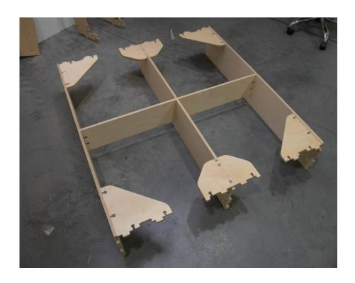
Step 5 Align the tabs and slots and attach the two End Panels using eight 5/16 x 1 1/4 Machine Screws and Nuts for each End Panel as shown.
