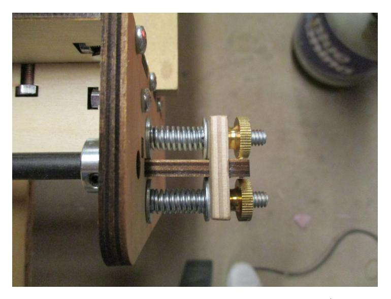
In a nutshell, I installed (2) screws, (4) washers, (2) springs, and (2) knurled knobs, for less than \$5, and using the parts that came with the machine in the first place, without interfering with the overall travel of the Y-gantry in the X direction.
