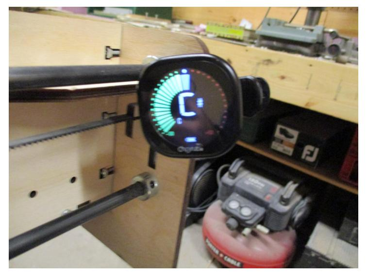
The only way I have to "measure" the tension in each belt is by sound.....I used one of my guitar tuners to adjust the "note" of each belt until each of them vibrate with the same frequency.
