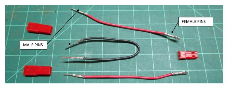
Crimp a male pins on one end of each red wire and both ends of the black wire.
