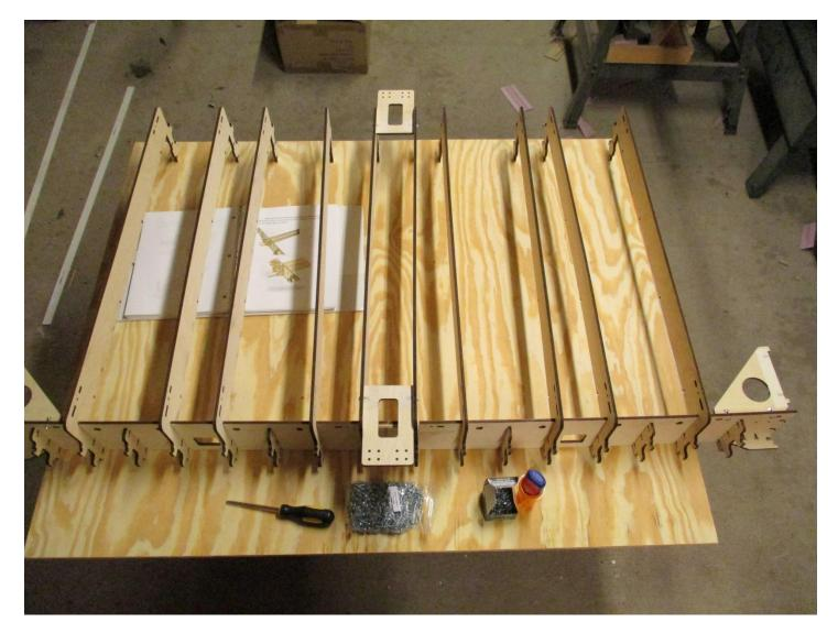
Now, turn the frame back over and GENTLY coax the other X5 Extended Side frame down onto the Mid Frames, aligning the tabs and slots. Secure each X4 Mid Frame to the X5 Side Frames with (2) M4x16 screws and nuts, starting with the X4 Mid Frame/X7 Wire Harness assembly, and again, working your way out to each end, alternating to each side of the middle frame. Make sure the Side frames are oriented correctly.
