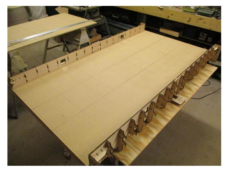
After locating the drilling centers, slide the spoil board into the frame and **CHECK THE ALIGNMENT AND THE HOLE CENTERS.**
