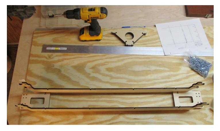
Locate and secure the lower (4) X8 Frame Corner Supports and the (4) upper X2 Frame Corner Braces as shown. Make sure the orientation matches what's shown in the manual.
