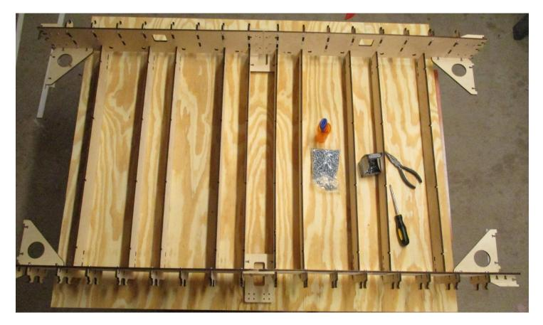
Locate, align, and attach the X6 Frame End Supports per the manual.
