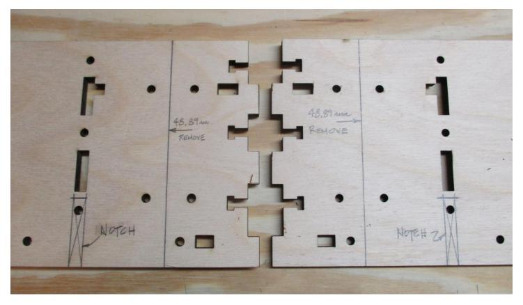
Remove 48.89 mm (1 15/16") from the "middle" ends of (4) X5 Frame Side Supports .....for a total of 97.78mm (3 7/8") Cut a notch to match the X4 Frame Mid Support as shown. **Do not drill the side frames just yet.**
