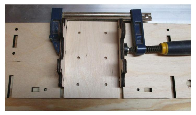
Secure (2) X1 Rail Supports with (4) M4x16 screws and nuts, and epoxy the drilled plywood plate between the rail supports. <u>Make sure the X5 frames are aligned exactly</u>. <u>Clamp securely</u>. I used Loctite 5 minute Epoxy. Let it cure completely. The X1's are temporary and used for alignment and fit. X4 Mid Supports will be added in their place. Make sure you don't epoxy X1's to the frame sides or the splice plate.
