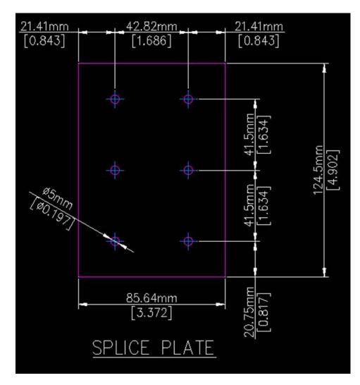
Make (2) Splice plates as shown out of 6mm Baltic Birch plywood (from BobsCNC)
