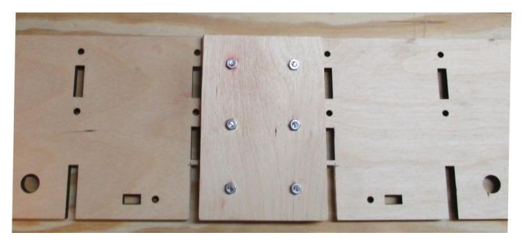
Drill the X-Frame side frames to match the splice plate and bolt together with (6) M4x16 screws and nuts. Tighten per the Evolution 4 assembly instructions (snug +  $1\frac{1}{2}$ ). Remember the Loctite Thread Lock
