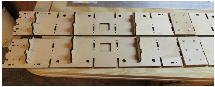
Assemble (2) X4 Mid Supports and (2) X7 Wire Harness supports as shown:
