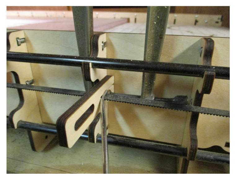
I cut the zip ties holding the belt in place and removed the screws of the X-rail Stop.
