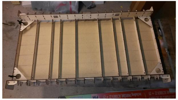
I chose to secure the spoil board at this point..I match drilled the spoil board and countersunk the holes to accept M4x16 flat head machine screws.
