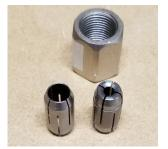
Quantum CNCs only include a 1/4" collet, so you'll need to purchase a 1/8" collet (or an adapter) if you want to use bits with smaller shanks. (right pic, Makita collets, showing a purchased 1/8" collet<sup>[1]</sup> along with the stock parts)
