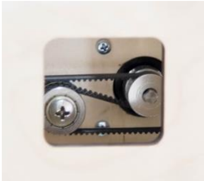
Finished Belt Routing viewed through the access port.
