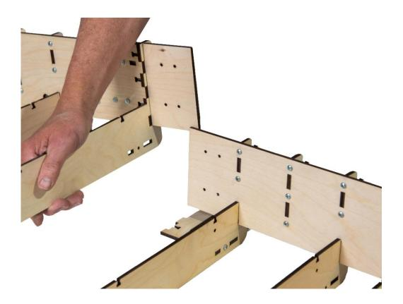
**Step 2** While aligning the components, make sure the tabs of the Wire Harness fit into the adjoining slots of the X Frame Mid Support. Secure the Coupling Plate with four M4 x 16 Screws and Locking Nuts and the Wire Harness Support with one M4 x 16 Screw and Nut. Repeat for the other side.
