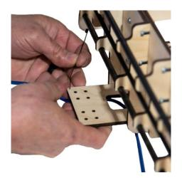
Step 7 Secure the Power Cords to the underside of the Wire Harness with Zip Ties as shown.
