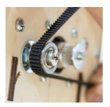
8f Loop the Belt over the Belt Pulley so that the Belt teeth engage the teeth of Pulley.
