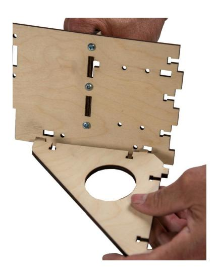
Step 5 Attach the Frame Corner Braces and secure to the Extension Frame Side with two M4 x 16 Screws and Nuts for each Brace.
