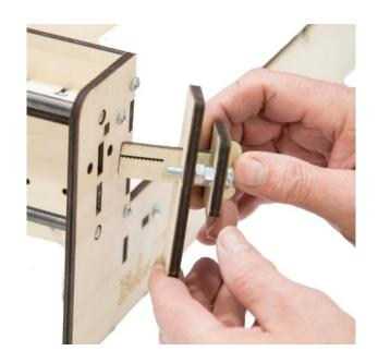
**9e** Insert the end of the Belt into the Belt Retainer. Be sure to seat the Belt completely in the Retainer as shown.
