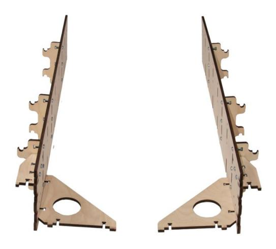
Step 6 Align the tabs of the X4 Frame Mid Supports with the slots in the Extension Frame Side Supports and secure with two M4 x 16 Screws and Nuts on each side. Repeat for the remaining 3 of the Frame Mid Supports.
