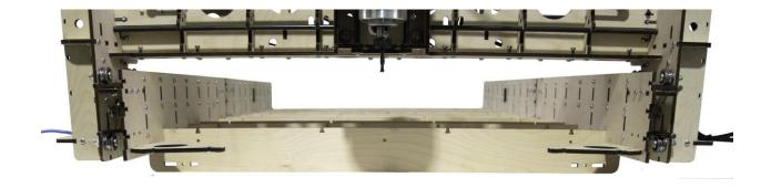
Step 5 Reinstall the Frame End Support and secure with twelve M4 x 16 Screws and Nuts.
