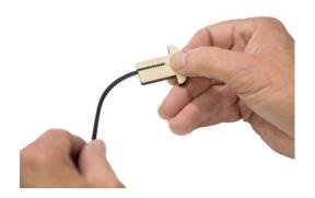
Next, thread the free end of the GT2 Belt through the Rail Stop (X3). NOTE: In the photo, the Rail Stop has been rotated so that the slot is oriented toward the bottom of the Rail Stop. Pull the belt through and insert the Short Belt Retainer through the Rail Stop as shown.
