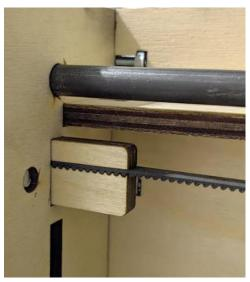
Step 10 Tighten the X1 and X2 Belts. Make sure the Nut closest to the Belt Adjusting Plate is tight. Using a 10mm wrench, hold the adjustment Nut and turn the machine screw to tighten the Belt. Be sure to adjust both Screws the same amount until the Belt is tight.
