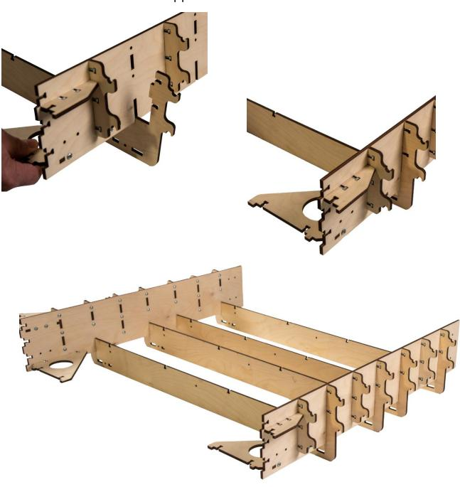
Step 7 Align the tabs of the X7 Wire Harness Supports with the slots in the Extension Frame Side Supports and secure with one M4 x 16 Screw and Nut each side.
