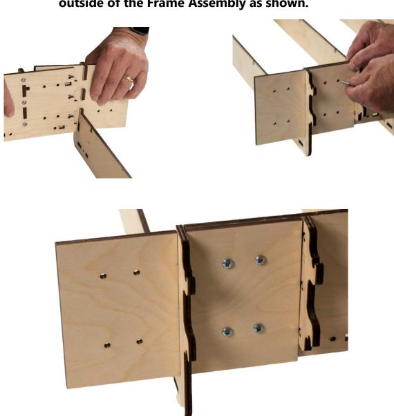
Step 3 Align the tabs of three X1 Rail Supports to slots of the EX5 Extension Frame Side Supports and secure each with three M4 16 Screws and Nuts.
