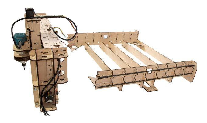
Step 8 Remove the four X Rails and discard. The X frame I now ready once the extension is built. Set aside t X frame for later assembly
