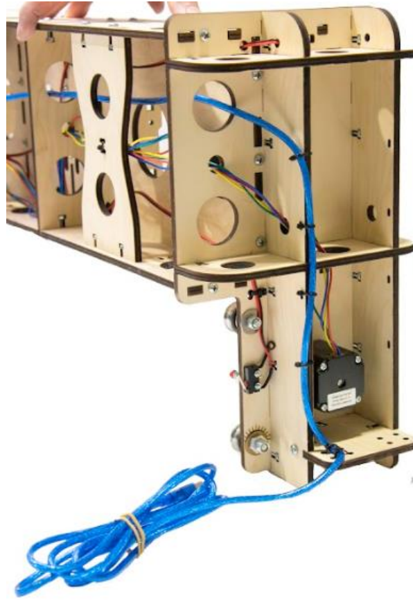
28f Wire Management: Bundle and secure the Stepper Motor Wires to the back of the Gantry Back Support with a Zip Tie as shown.
